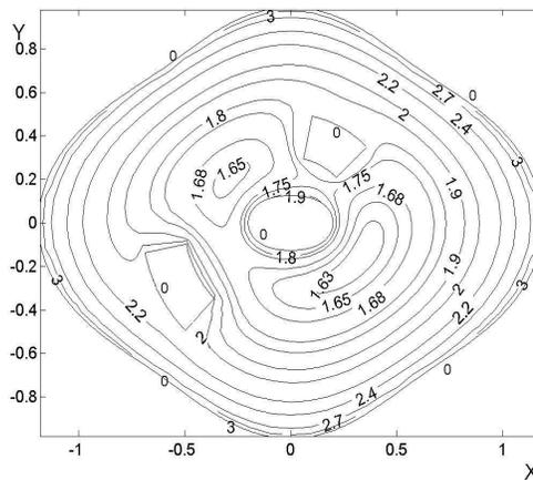
Figure 4. Contours of equal pressure under the punch with the multiply-connected base
