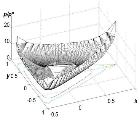
Figure 2. The normal pressure distribution under the punch with the base bounded by the triangles
