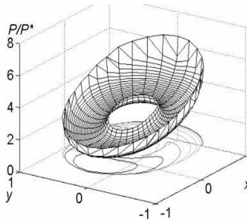
Figure 1. The normal pressure distribution under the punch with the base bounded by the Booth lemniscates
