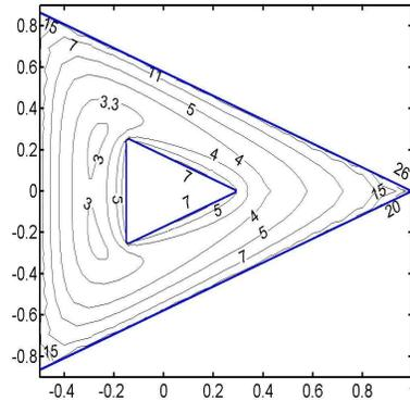
Figure 3. Contours of equal pressure under the punch with the base bounded by the triangles
